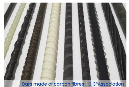
Bars made of carbon fibres | © C 3 Association
